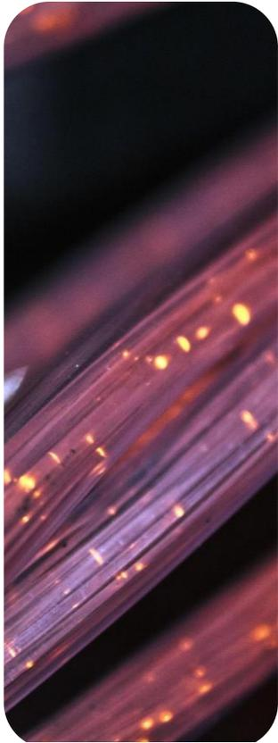
Covert fiber-optic cables are deployed along your perimeter – buried underground or mounted on fences and walls – forming an invisible detection grid. A centrally located *interrogator* unit continuously sends light pulses through the fibers and monitors the return signal.
